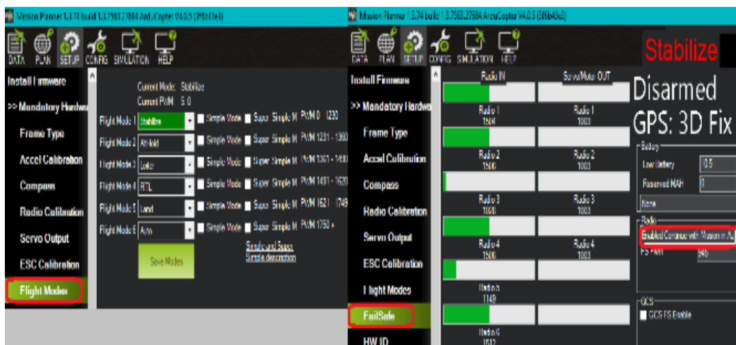
Figure 8: Setting flight modes and FailSafe
