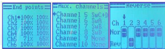
Figure 7: Setting parameters on the FlySky FS-i6 operation panel for the formation of flight modes
